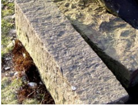
A partially finished kerbstone showing the dressing marks on the top surface.
